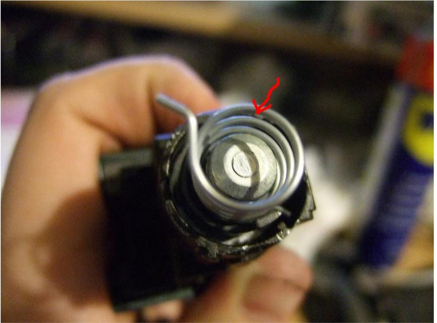
**Step11** : This is where the spring goes in, when you are pushing the paddle down you need to twist it put the other end of the spring behind the catch roughly in the position of the arrow.
