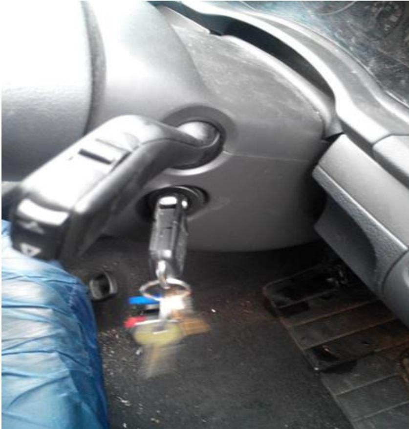
When both wipers have been changed, turn the keys to accessories live position, push down once more on the wiper stalk and the wipers will return to their normal positions.
