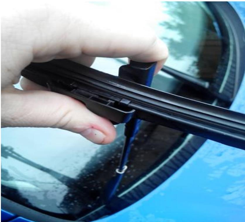
Installation is just a case of fitting the new pin on. Remember to measure up the wiper blades against your old ones to find out which is which. The wiper on the driver's side is 600mm; the driver's side wiper is always the longest due to covering the biggest area of visibility as required
