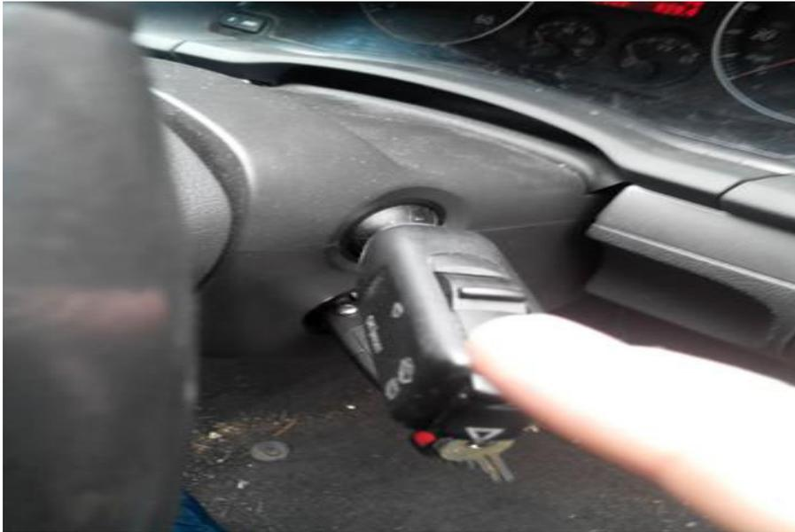
When the keys have been removed push down on the wiper stalk, you will then see the wiper blades move up and stay there. The wipers are now in the position for the wiper blades to be changed without affecting or colliding with the bonnet itself.
