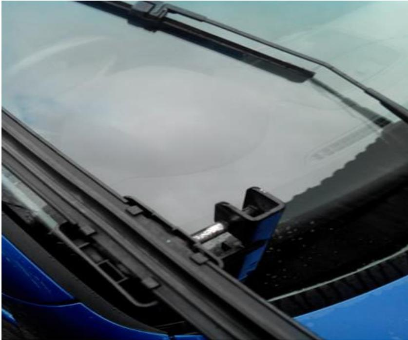
You then pull the rod away from the stalk after rotating it, it's held on a pin, picture as follows. Keep pulling and it will be removed
