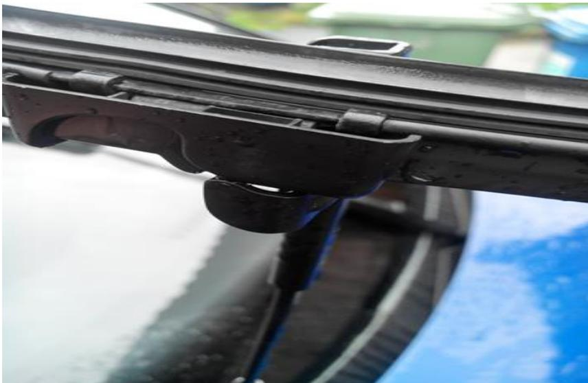
On my specific model the wiper blades are side loading. Which means they're on a small rod held in place by a pin. To change the wiper blades on a the Golf MK5 you rotate the wiper blade backwards away from the screen after you lift it up as such
